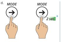
\* If the pallet truck is already in count mode (sampling enabled), press the MODE button for two seconds for re-sampling.
