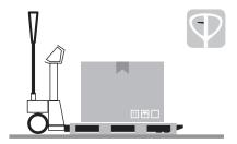
The pallet truck is equipped with a dual-function tiller: traction or manoeuvre and hydraulic lift. **NOTE:** raise or lower the truck ONLY when stationary.
