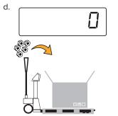
Load the desired reference quantity (e.g. 5 pieces). For a correct sampling, the reference quantity must have a weight of at least 0.1% of the maximum scale capacity.
