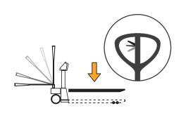
h. Using the control lever, the downwards movement can be carried out from any tiller position.
