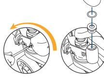
Remove the protective casing, the seal and the cap.
